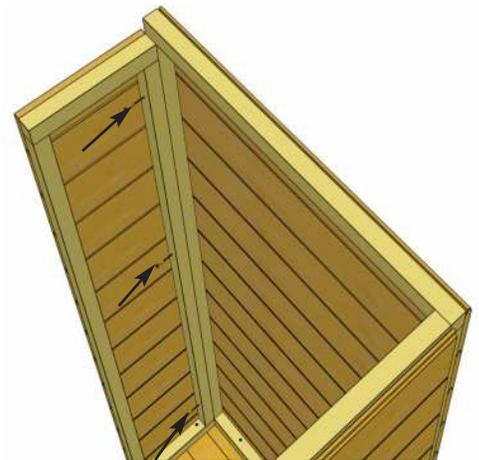
**10.** Align Wall framing flush with outside of Floor framing. When correctly positioned, secure Bottom Wall Plate to Floor with **2 - 2 1/2" Brown Screws**. Attach vertical Wall framings together at top, middle and bottom with **3 - 2 1/2" Brown Screws**.
