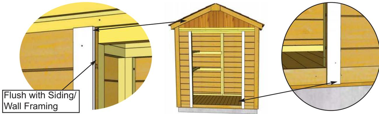
**56.** Locate 2 **Vertical Door Frame Trims**. Position on Front Narrow Wall flush with Wall siding/ framing and underneath Front Header Filler Strip. Attach with **6 - 1 1/2" Finishing Nails**.
