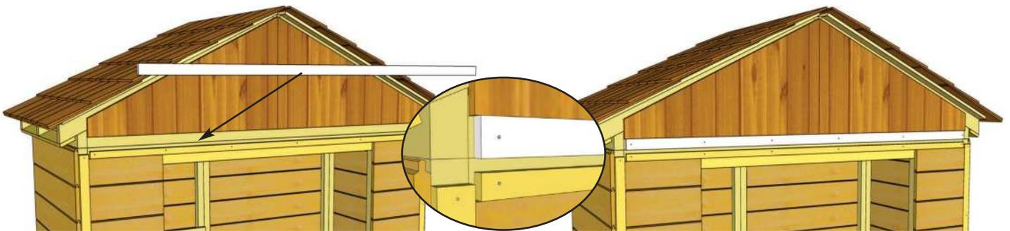
**44.** Locate **Front Top Plate Filler Strip**. Position Front Top Plate Filler Strip onto Front Top Plate. Evenly space from side to side. Secure with **6 - 1 1/2" Finishing Nails** into Front Top Plate.
