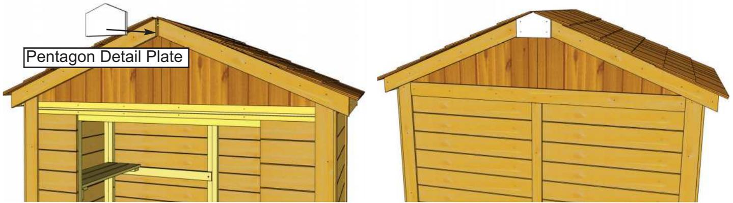
**55.** Attach **Pentagon Detail Plates** where Front and Rear Fascia Trims meet at the peak. Secure with **4 - 1 1/2" Finishing Nails** per piece.
