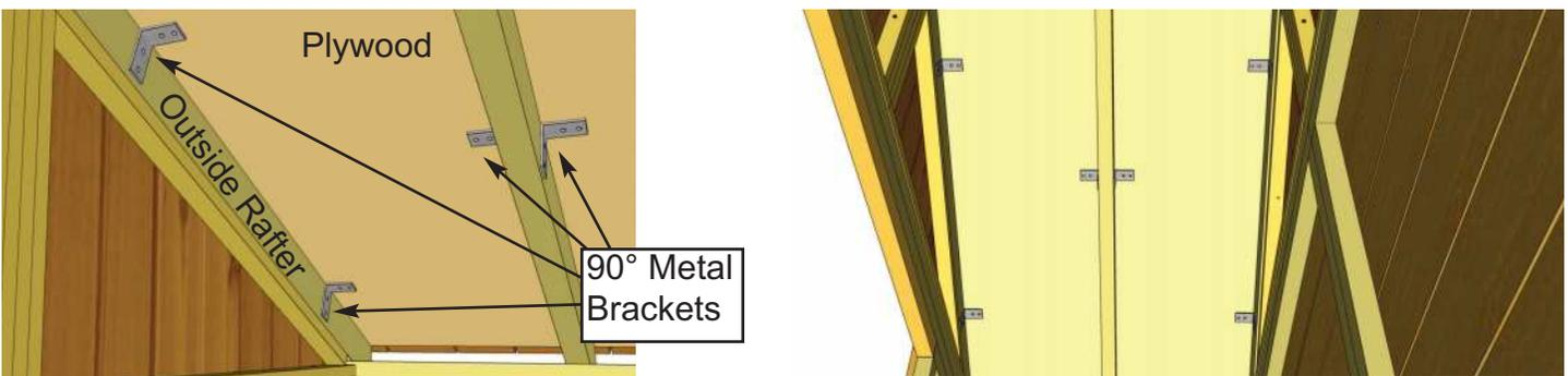
**37.** Inside the shed, position **6 - 90° Metal Brackets** onto the Roof plywood and Rafters and secure with **4 - 3/4" Silver Screws** each Bracket. For each Roof Panel, 4 - 90° Metal Brackets will be used for the outside Rafters and 2 - 90° Metal Brackets will be used to secure the middle Rafter.
