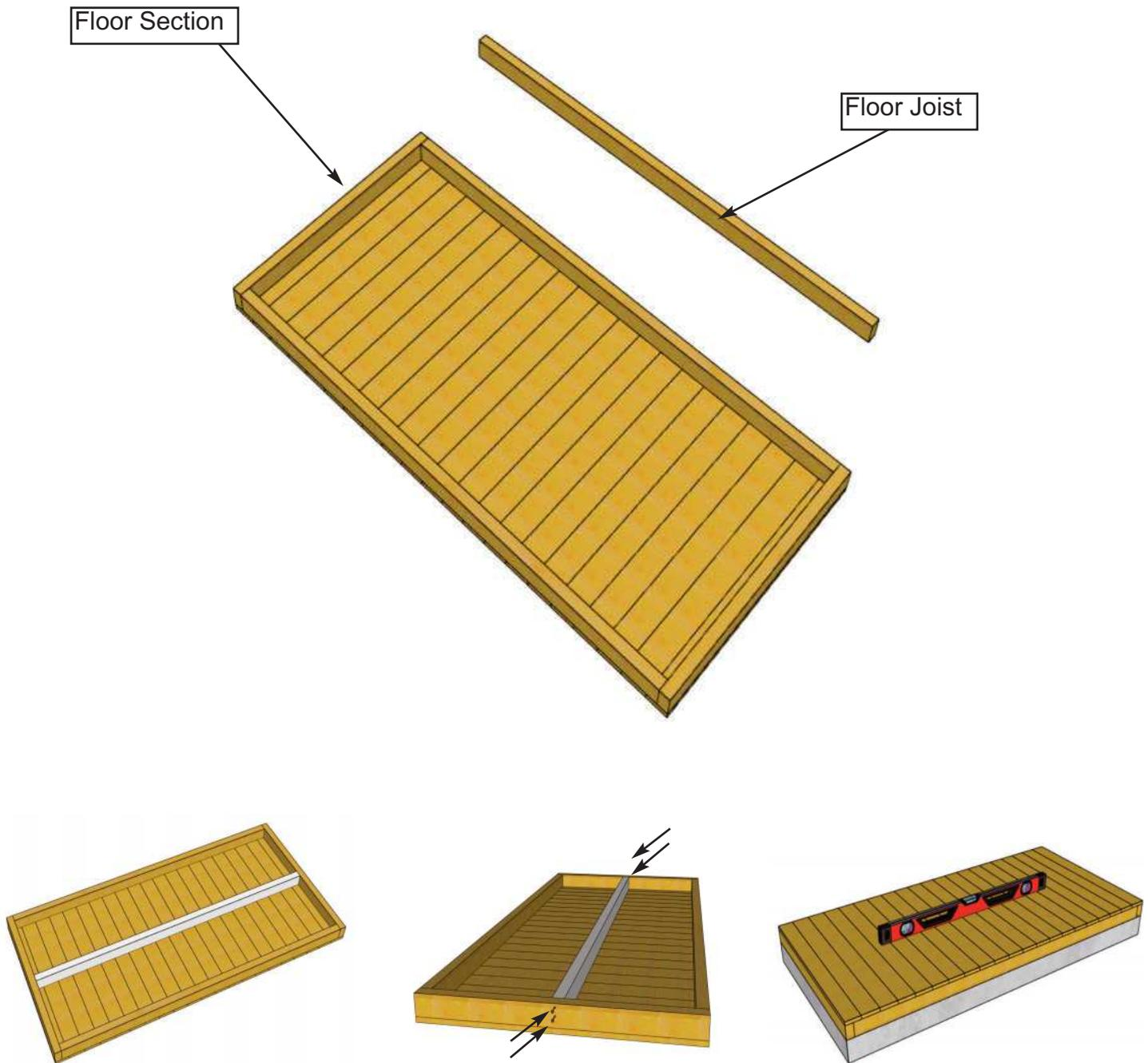
**1.** Locate **Floor Joist** and position at center of **Floor Section** and flush with framing as illustrated above. Attach with **2 - 2 1/2" Brown Screws** per end. Flip over and lay Floor Section on a level foundation only. Patio Stones or a Concrete Slab both make excellent foundations. (See Page 3 for more information on foundations). Use a level to confirm and shim Floor Joist as required.
