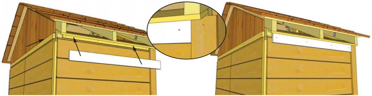
**48.** Locate **Upper Horizontal Side Wall Trim** and align tight against Front Side Corner Trim. Attach to Upper Horizontal Side Wall Filler Trim with **4 - 1 1/2" Finishing Nails**.
