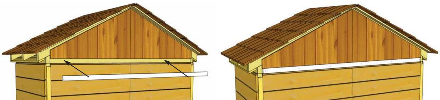
**45.** Locate **Rear Top Plate Filler Strip**. Position between Rear Walls and Rear Gable. Evenly space from side to side. Secure with **6 - 1 1/2" Finishing Nails** into Rear Top Plate.
