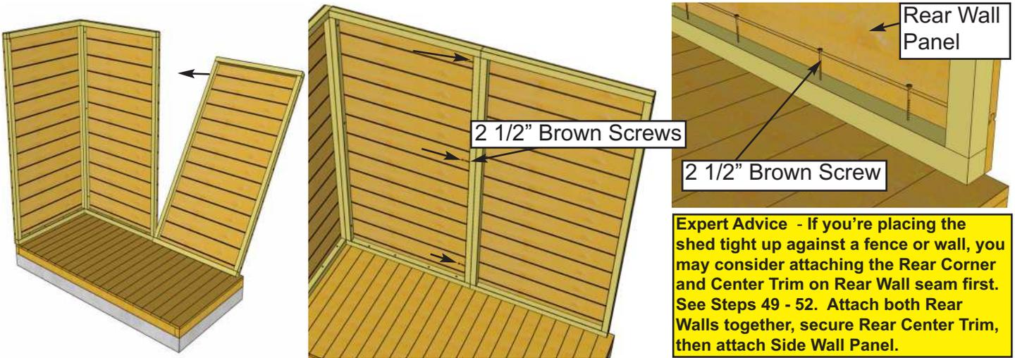
**7.** Position second **Rear Wall Panel** on Floor as per **Step 6**. Attach Wall frames together at top, middle and bottom with **3 - 2 1/2" Brown Screws**. Secure Bottom Wall Plate to floor with **4 - 2 1/2" Brown Screws**. **Important: Confirm Siding on Rear Wall Panels are aligned.**
