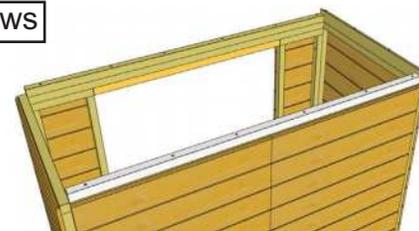
**18.** Locate **Rear Top Plate** and place on top of Rear Walls. With Rear Top Plate positioned evenly and flush against Rear Wall framing, secure using **6 - 2 1/2" Brown Screws** screwing down from the top of Rear Top Plate down into the Rear Wall top plates.
