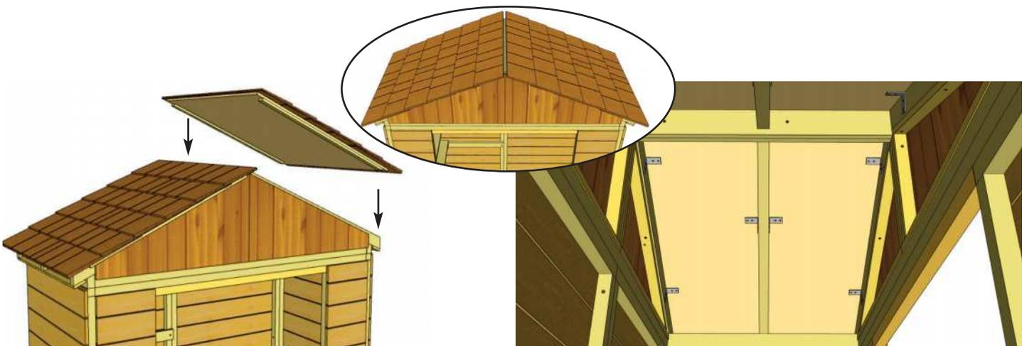
**38.** Place second Roof Panel on Rafters and secure inside as per **Steps 36 - 37.**
