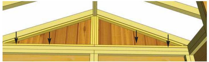
**33.** With both Ridge Boards connected, completely secure Gable framing to Walls and Rafters. Use **3 - 2" Brown Screws** per Rafter. Use an additional **4 - 2" Brown Screws** to secure Gable to Wall. **Note:** you may have to remove the 2 temporary screws in Gable from Step 21 and reposition Gable for best fit prior to completing Gable attachment.
