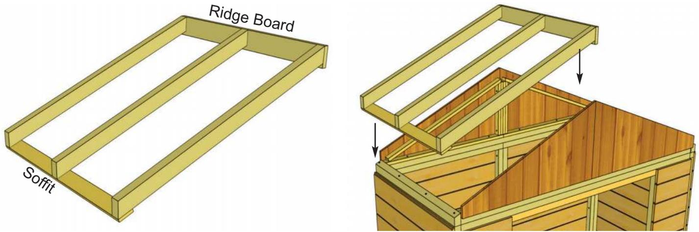
**28.** Flip Rafter section over so Soffit is facing down. Starting with one side, lift completed Rafter Section up and place on Gable framing.
