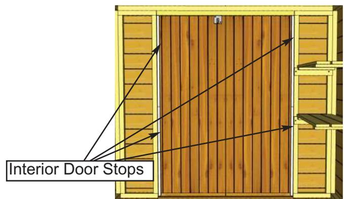
**69.** Attach top Interior Door Stop as per **Step 68** and then complete the opposite side.
