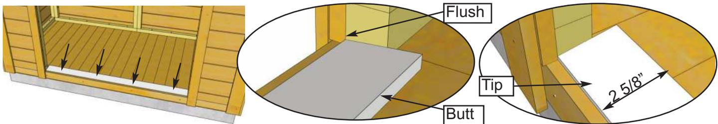
**57.** Locate **Door Threshold** and position on Floor at the opening. Align tip of the bevel flush with the outside of Bottom Wall Plate. Attach with **4 - 1 1/4" Brown Screws**.
