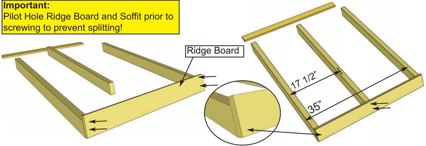
**25.** Starting with first Rafter section, attach Ridge Board to ends of both outside rafters with **2 - 2" Brown Screws** per end. Drill 1/8" pilot holes in Ridge Board to prevent splitting. Measure and position interior Rafter as illustrated. When positioned correctly, attach Ridge Board to remaining Rafter with **2 - 2" Brown Screws**.
