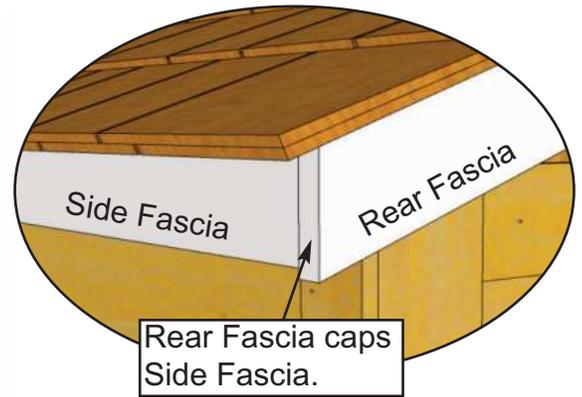
**53.** Position **Rear Fascia** (angle cut on ends) and **Side Fascia** (square cut ends) in corner. Line Fascia up so Rear Fascia caps Side Fascia. Attach Rear Fascia to Nailing Strip with **6 - 1 1/2" Finishing Nails** and Side Fascia to ends of Rafters with **6 - 1 1/2" Finishing Nails**. Gap where Fascia boards come together at peak will be covered in **Step 55**. Do a dry run using Side Fascia to help you correctly position before attaching.
