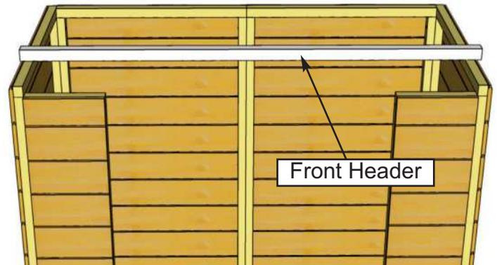
**12.** Locate **Front Header** and place on top of Front Narrow Wall framings.
