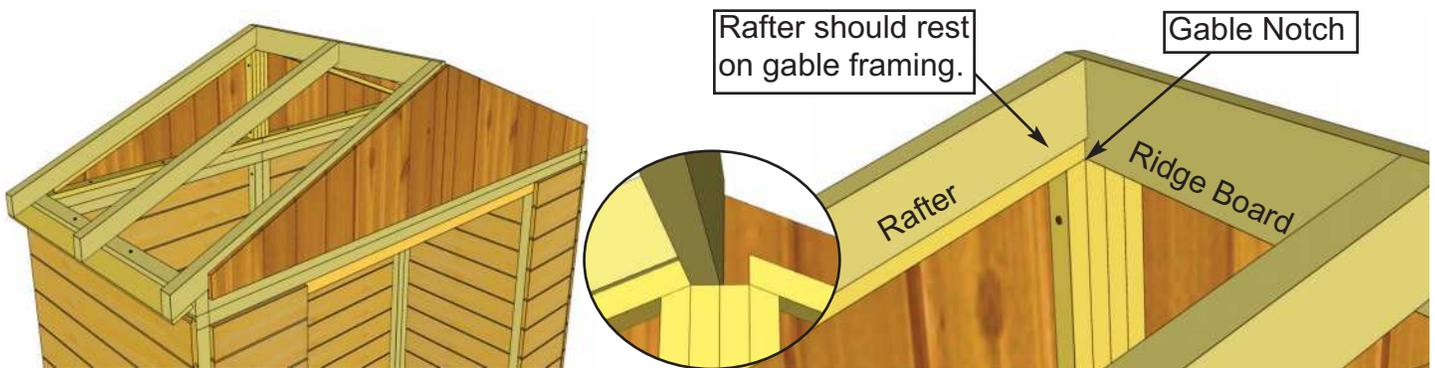
**29.** Slide Rafter section up on Gable framing until bottom of Ridge Board slips into Gable notch.
