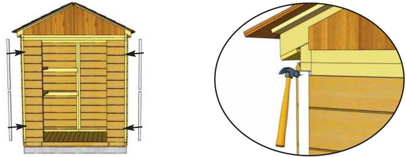
**41.** Locate 4 **Front Filler Trims**. Filler trim will be covered by Corner Trim in **Step 47**. Attach in each front corner with **3 - 1 1/2" Finishing Nails** per piece.
