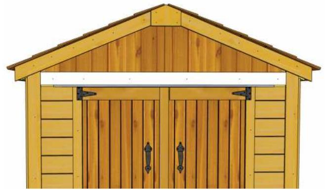
**70.** Locate **Front Horizontal Trim** and **Metal Drip Edge**. Position Metal Drip Edge behind Door Trim. Evenly space from side to side. While holding down both Metal Drip Edge and Front Horizontal Trim, secure with **6 - 1 1/2" Finishing Nails** into Front Header Filler Strip.
