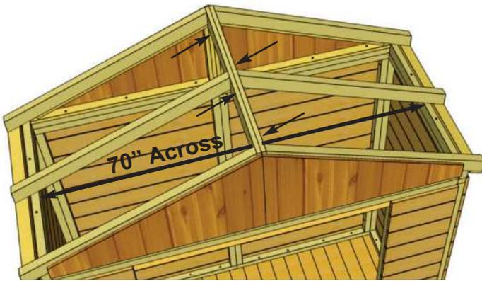
**32.** At the peak, align Ridge Boards so they are flush together and secure them with **4 - 1 1/4" Brown Screws**. **Important:** If there is a gap between Ridge Boards, have a helper push the Side Walls closer together from outside. Walls should be 70" apart at top from inside of Wall plate to opposite Wall plate.
