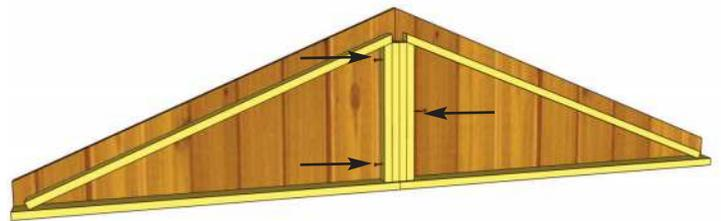
**20.** Locate **Front/Rear Gables** and align Gable framing and siding together. Screw center Gable framing of each piece together with **3 - 2 1/2" Brown Screws**.
