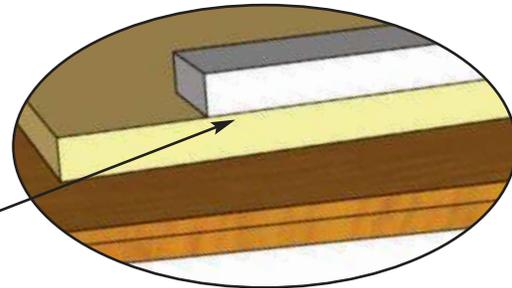
**35.** Carefully flip **Cedar Shingle Roof Panels** over so plywood is facing up. Attach **Roof Nailing Strips** onto outside of each panel flush with plywood. Attach with **3 - 1 1/4" Brown Screws** evenly spaced. Nailing Strips provide for a greater nailing surface later when you attach Front/Rear Fascia Trim.
