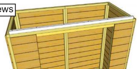
**16.** Locate **Front Top Plate** and place on top of Front Header. With Front Top Plate positioned evenly and flush against Front Header, secure using **6 - 2 1/2" Brown Screws** screwing down from the top of Front Top Plate down into Front Header.
