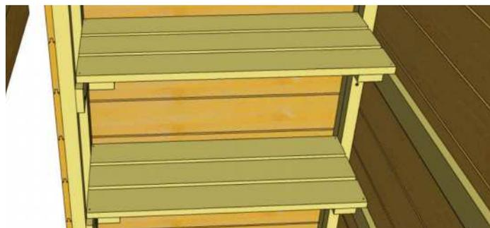
**23.** Place **Storage Shelf** on top of supports and secure with **4 - 1 1/2" Finishing Nails**. Complete 2nd Shelf (if desired) as per **Steps 22 & 23**.
