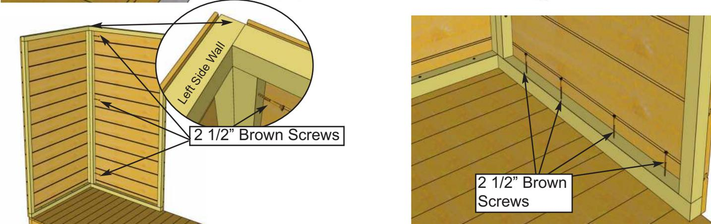
**6.** When Side and Rear Walls are aligned in corner correctly, Wall framings will be flush. Attach Wall framings together with **3 - 2 1/2" Brown Screws**. Secure Bottom Wall Plate to Floor with **4 - 2 1/2" Brown Screws**.
