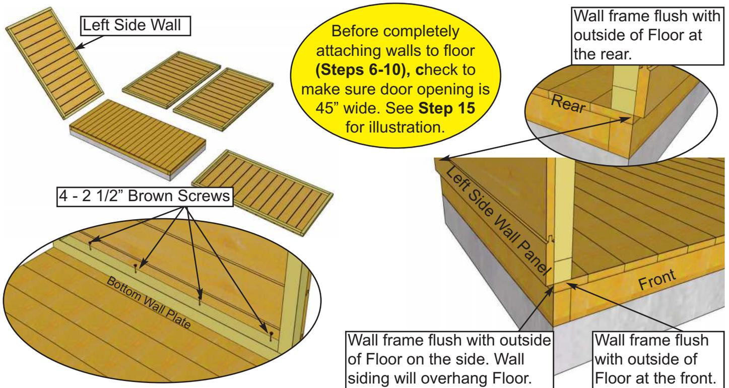
**4.** Starting with **Left Side Wall**, lift up and position so framing is flush with Floor at both front and rear of shed. Make sure Wall frame is flush with outside of Floor on the side. When Wall is positioned correctly, secure Bottom Wall Plate to Floor with **4 - 2 1/2" Brown Screws**.
