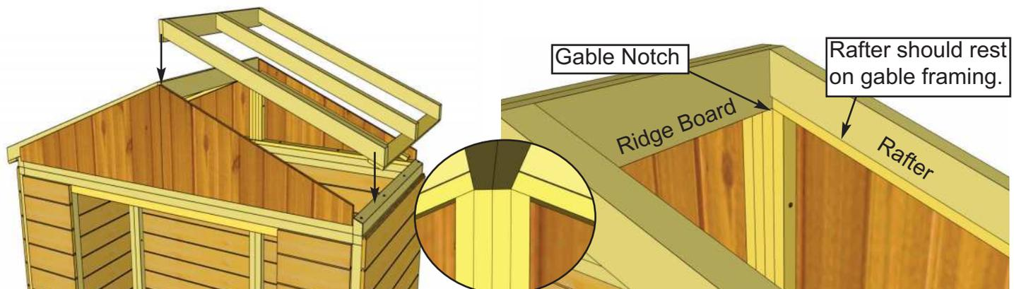
**31.** Place second completed Rafter section on Gable framing as per **Steps 28 - 29.**
