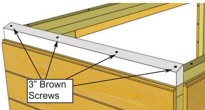
**19.** Complete opposite **Side Wall Top Plate** positioning and attachment as per **Step 17**.
