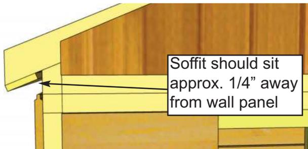
**30.** When Rafter section is correctly positioned, outside rafters will sit equally on Gable framing and soffit will sit approximately 1/4" away from wall panels.
