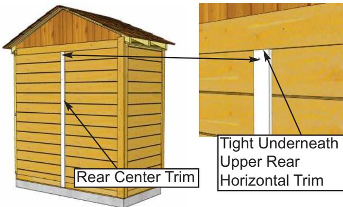
**51.** Locate **Rear Center Trim**. Align tight against Upper Rear Horizontal Trim and attach with **6 - 1 1/2" Finishing Nails**.
