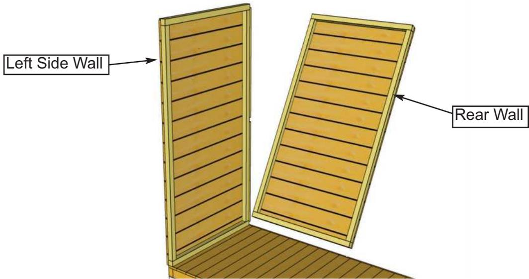
**5.** With your helper holding the Side Wall Panel, position a **Rear Wall Panel** in rear corner. **Important: Align Wall Framing Flush with Floor Framing.**
