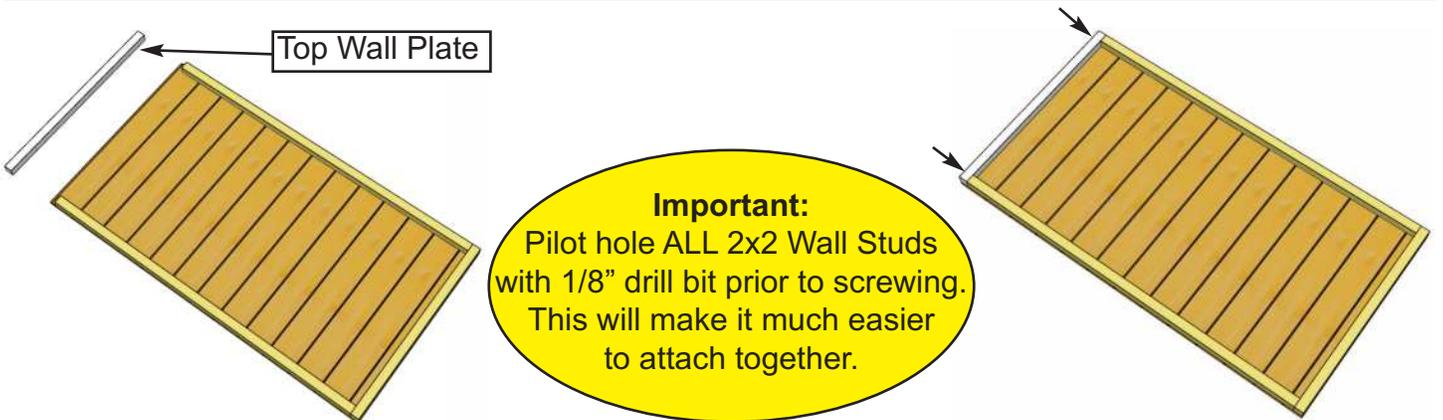
**2.** For each **Rear and Side Wall Panel**, carefully lay Panel face down. Position and attach a **Top Wall Plate** to top of wall studs of each Wall Panel with **2 - 2 1/2" Brown Screws**. Position so Plates are flush with framing.
