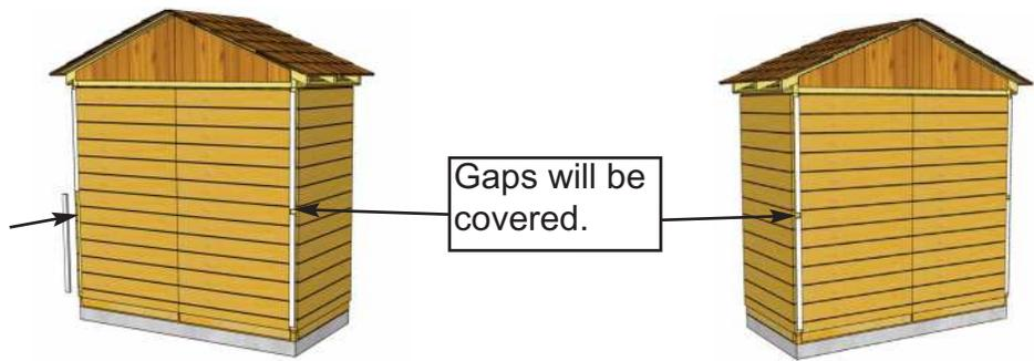
**42.** Position and attach **Rear Filler Trims** in the rear as per **Step 41**.
