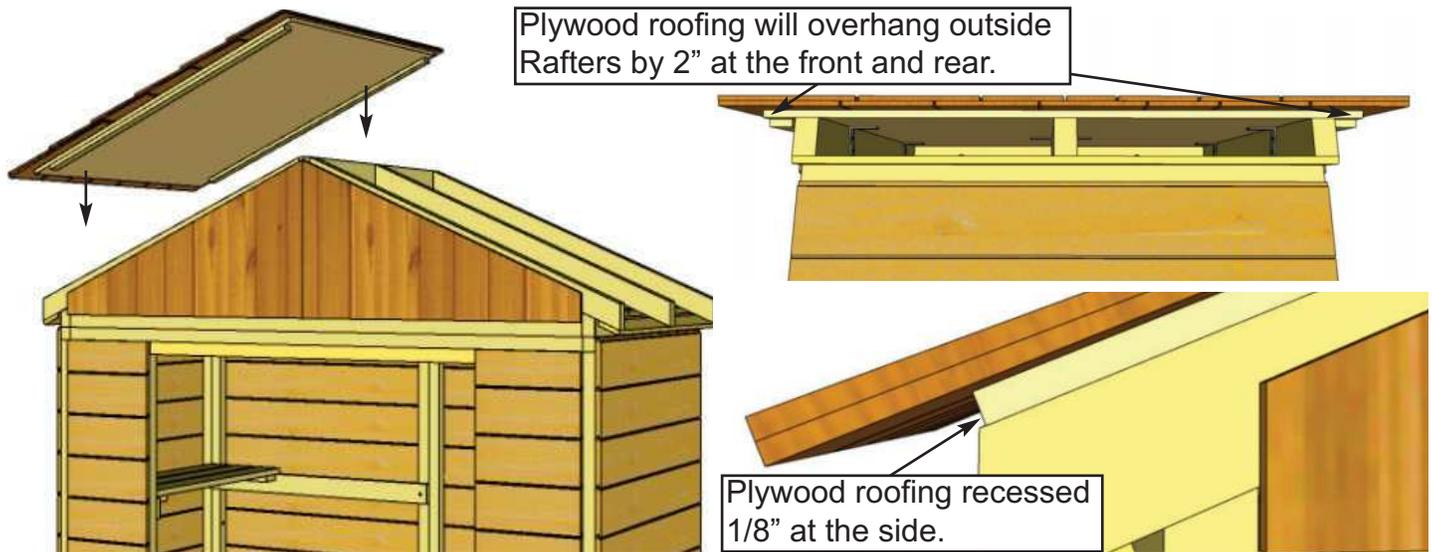
**36.** Lift up first **Cedar Shingle Roof Panel** and place on Rafters. At the front and rear, plywood roofing should overhang Rafters by 2" and recessed 1/8" back from Rafters at the side.
