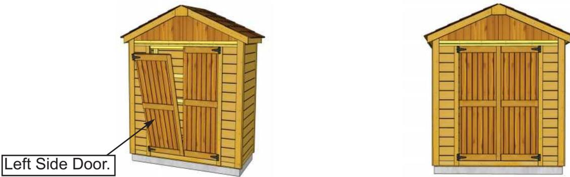
**61.** Position Left Side Door (with Flange) as per **Step 60**. Once again, use only **1 - 2" Black Headed Screw** per Hinge initially to secure door to Vertical Door Frame Trim.
