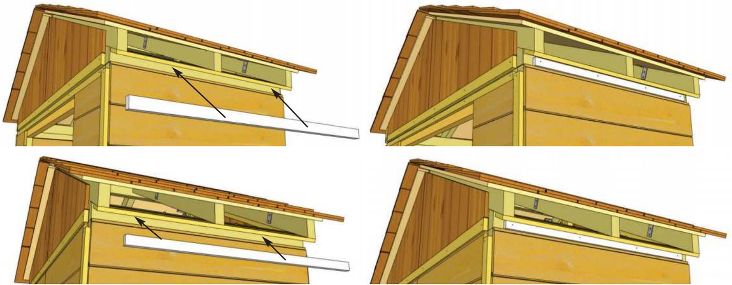
**46.** Locate an **Upper Horizontal Side Wall Filler Trim**. Position on Side Wall Top Plate. Evenly space from side to side. Secure with 4 - 1 1/2" **Finishing Nails** into Side Wall Top Plate. Complete opposite side with same positioning and attachment.
