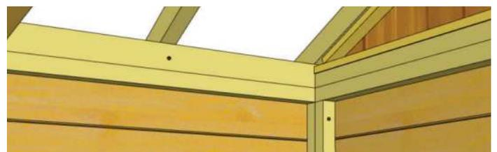
**34.** Attach middle Rafter to Side Wall Top Plate inside of shed using **1 - 2 1/2" Brown Screws** angled upward. Complete attachment of opposite middle Rafter.
