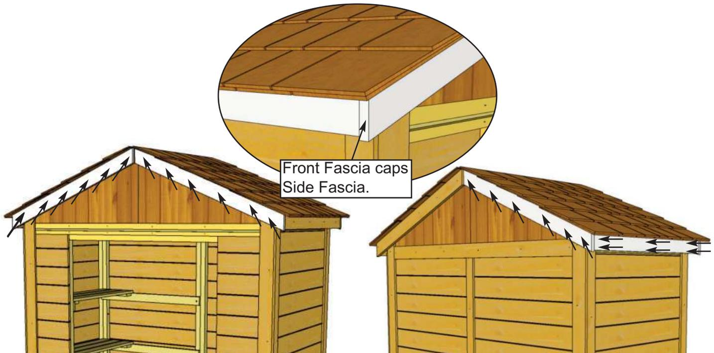
**54.** Attach remaining Front and Rear Fascia to Nailing Strips and attach remaining Side Fascia to Rafter ends as per Step 53.
