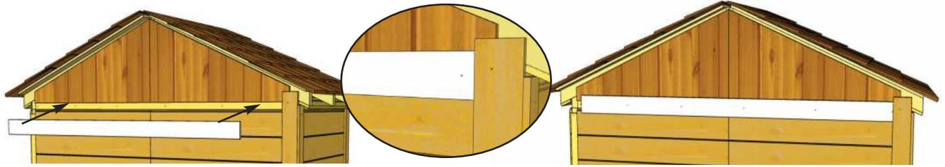
**50.** Locate **Upper Rear Horizontal Trim** and align tight against Rear Wide Corner Trim. Attach to Rear Top Plate Filler Strip with **6 - 1 1/2" Finishing Nails**.
