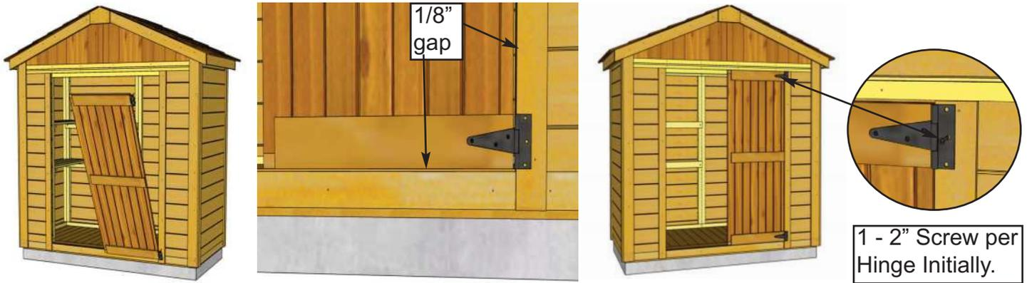
**60.** Starting with Right Door first, lift and position Door in opening. Leave a 1/8" gap on right side and 1/8" gap on the bottom. Use a **Cedar Shingle Shim** to shim the Door at bottom to help position door evenly. When Door is aligned correctly, screw Hinge into Vertical Door Frame Trim with **1 - 2" Black Headed Screw**. Use only 1 screw initially per Hinge until both Door alignments are confirmed. Drill pilot holes to prevent wood from splitting.
