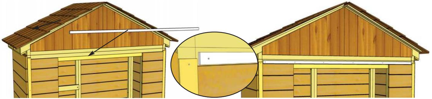
**43.** Locate **Front Header Filler Strip**. Position Front Header Filler Strip onto Front Header. Evenly space from side to side. Secure with **6 - 1 1/2" Finishing Nails** into Front Header.
