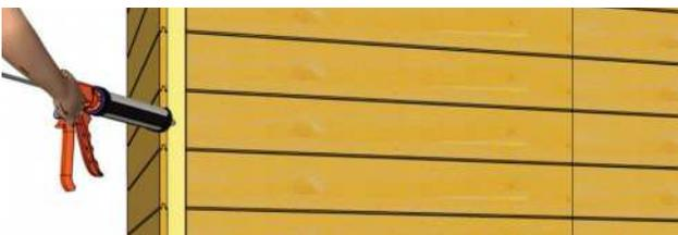
**39.** Check the wall seams for visible gaps prior to attaching Filler Trim and apply caulk where needed. Caulking gaps will help prevent moisture from entering and will help the longevity of your shed. **Caulking not included in kit.**
