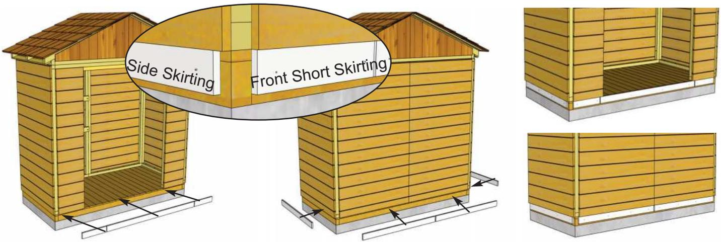
**40.** Locate **Lower Front Skirting (2 Short and 1 Long)**. Skirting will hide floor framing. Gaps will be covered by Wide Trim pieces later. Attach 2 Lower Short Front Skirting pieces with **2 - 1 1/2" Finishing Nails** per piece. Attach Lower Front Long Skirting with **4 - 1 1/2" Finishing Nails**. Locate **Lower Side and Rear Skirting** and attach with **4 - 1 1/2" Finishing Nails** per piece.
