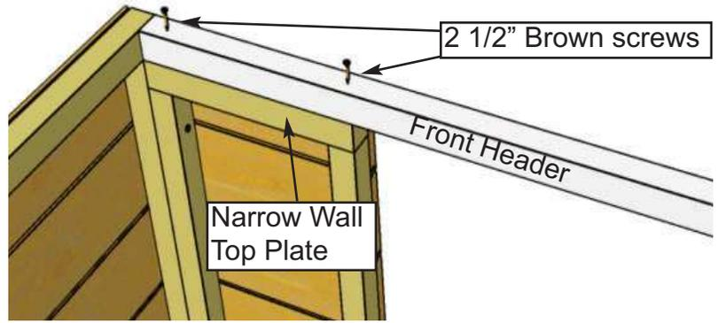
**13.** With Front Header positioned evenly on Narrow Wall top plates and flush against Side Wall top framing, secure using **4 - 2 1/2" Brown Screws** screwing down from the top of Front Header down into the upper Narrow Wall plates. Have your helper push side walls against end of Front Header to achieve tight fit if possible.
