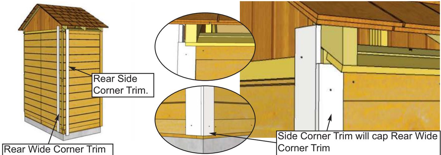
**49.** Locate a **Side Corner Trim** and **Rear Wide Corner Trim** and position both Trims up underneath Cedar Roof and Soffit. Align Rear Wide Corner Trim with bottom of Side Corner Trim. Side Corner Trim will cap Rear Wide Corner Trim. When correctly aligned, attach each piece with **6 - 1 1/2" Finishing Nails**.
