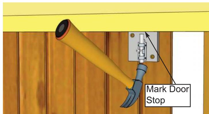
**66.** Position the **Interior Silver Barrel Bolt** on the Plywood Spacer and attach with **4 - 3/4" Silver Screws**. Tap Silver Barrel Bolt with hammer on underside of Interior Door Header to mark location.
