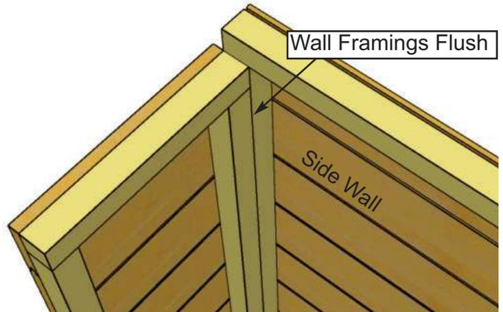
**9.** Locate **Front Narrow Walls** and position Wall framing flush with Side Wall framing in corner. **Important: Make sure Narrow Wall is positioned right side up.**
