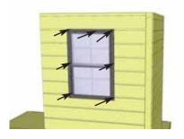
**11a.** Position Window Trim around window doing a dry run first and attach with  $4 - 1 \frac{1}{2}$  finishing nails per piece. The window kit trim pack =  $1 \times 24 \frac{1}{16}$  = top /  $3 \times 23$  = sides and bottom. Window trim has a small dado on reverse face. Outside flange of window will roughly sit in the dado to give a better fit.
