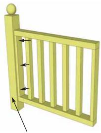
Use Rail Support Block (3 1/2" high) from bottom of post to align rail. Attach rail to post with 3 - 2" screws.
