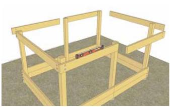
**8.** Measure 48" from the ground to establish the height of the top Front Girder. Level Girder and attach as per **Step 3**. Lay out and secure remaining top & rear Girders as per **Step 4 & 5**.
