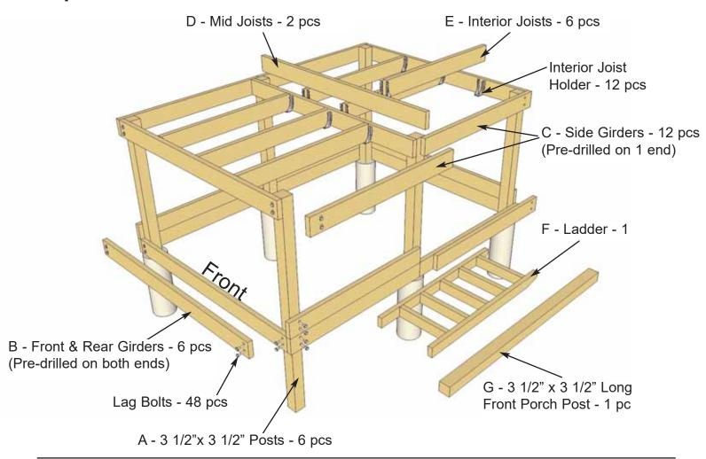
1. Before you receive your Playhouse, clear the construction area. Remove all debris; roots, grass, rocks, etc. Dig holes for a 10" diameter **Concrete**Form (Sonotube) according to the illustration below. Concrete forms holes should be at least 15" in diameter and approximately 18" to 24" deep. The illustrations to right and below shows the exact center-to-center position of each post as it will be positioned in the sonotube.
