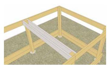
**10.** Position and attach Mid Joists (D) to mid Post using 4 - 3" screws per piece. Make sure Mid Joists are flush with Girders. Complete both Mid Joist attachments.
