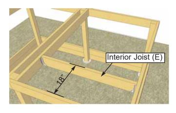
**11.** Measure 18" from end of Mid Joist to find the center of the Interior Joist Hanger. Position Interior Joist (E) in Hanger and attach Hanger to Mid Joist and Front or Rear Girder with 4 - 1 1/4". Make sure Interior Joist sits flush with top of Mid Joists and Girders prior to attaching.
