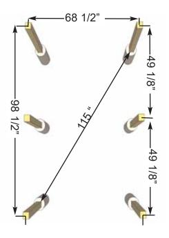
Post height may vary depending on the depth of your holes. Once concrete has been poured and curred in **Step 2**, measure and trim each post to correct height.
