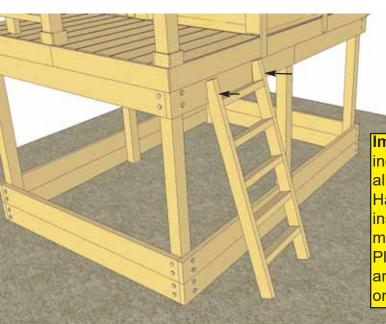
**15.** Attach Ladder (F) to side opening using 2 - 3" screws. Be sure to counter sink screws holes so screws do not pertrude out. Make sure gound is level so ladder is properly grounded.
