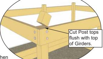
**9.** Complete all Top, Rear and Side Girder attachments. When complete, Post tops may need to be trimmed off so they are flush with tops of Girders. Use handsaw and be very careful.
