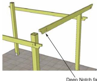
**5.** Locate Girder with Deep Notch on Bottom (C) and lift up between both completed Post/Girder Assembly's.
