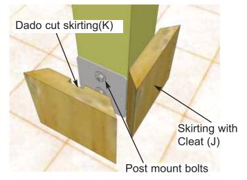
**24.** Locate all Post Skirting pieces. Position 2 post skirtings around the base of post as shown above. Use 1 Post Skirting with Cleat - 1 1/2" x 9" x 7 1/4" (Part J) and a Post Skirting with Dado Cut - 1 1/2" x 9" x 7 1/4" (Part K) initially. Cleat piece should be aligned opposite post mount hardware and dado piece aligned with post mount bolts (hardware).
