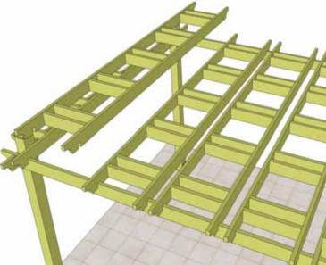
**16.** Set all remaining Ladder Sections in place on Girder spacing each **approximately** 5 1/2" apart.
