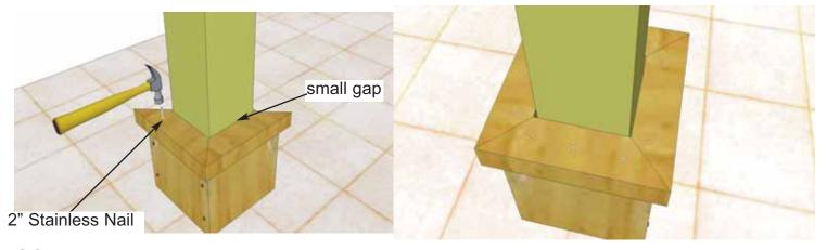
**26.** Position **Post Skirting Caps - 1 1/2" x 2 1/2" x 10 5/8" (Part L)** on top of skirting unit and against post. Do a dry run first to confirm fit. There will be a small gap between post and inside of cap. Attach caps down into skirting tops with **3 - 2 1/2" Stainless Steel Finishing Nails** per piece. Complete remaining post skirtings.
