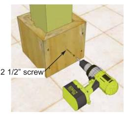
**25.** With your helpers assistance, screw Part J & K pieces together with 2 - 2" screws at pre-drilled locations. Make sure pieces are aligned on edges and top and bottom. Cleated skirting piece are pre-drilled. Complete remaining skirting pieces around the post. Position skirting unit evenly around post. Secure to post by screwing 1 - 2 1/2" screw into the center of each cleated skirting piece (J).
