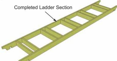
**13.** Complete all four Ladder Sections on the ground prior to moving to **Step 14**.
