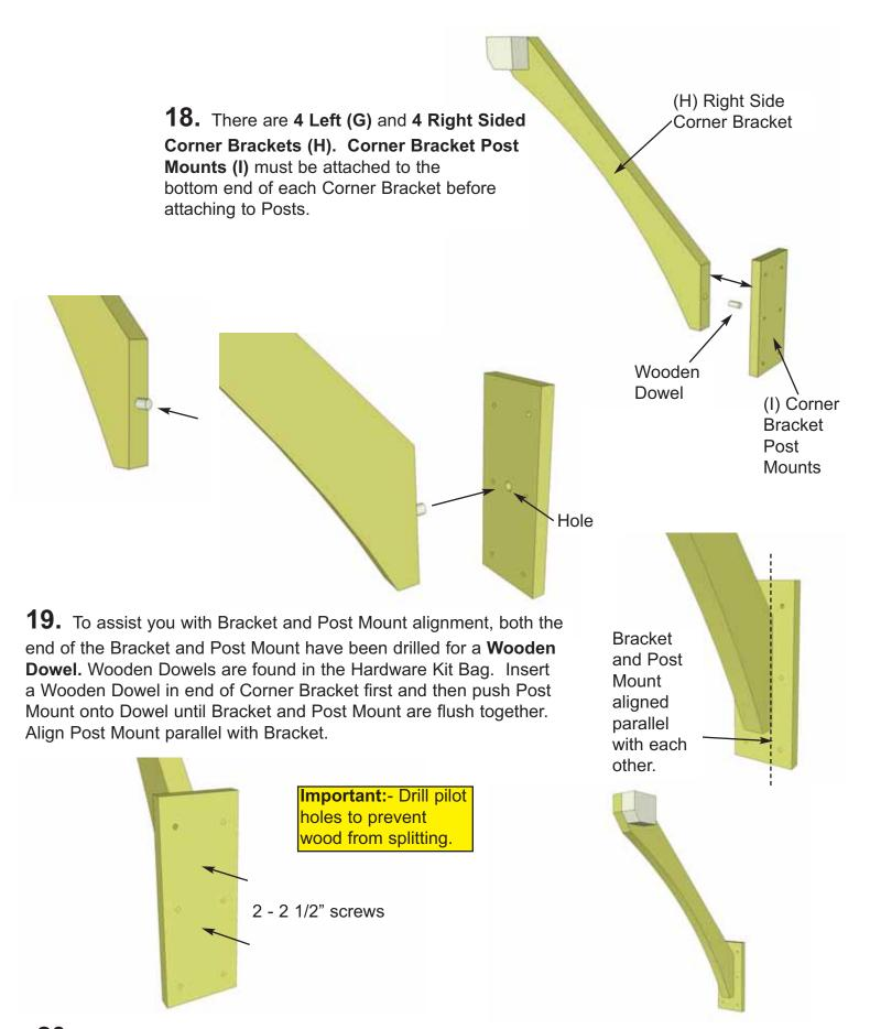
**20.** With Bracket and Post Mount correctly aligned, screw Post Mount to Bracket with 2 - 2 1/2" screws. **Important- Drill pilot holes in Post Mounts and Bracket to prevent wood from splitting!** Complete all remaining Brackets/Post Mount connections.
