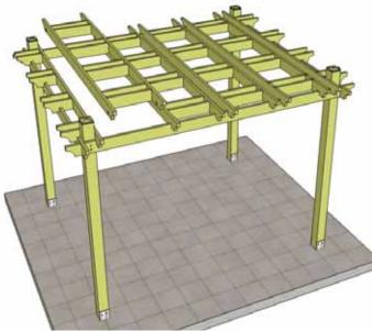
**16.** Set all remaining Ladder Sections in place on Girder spacing each approximately 5 1/2" apart.
