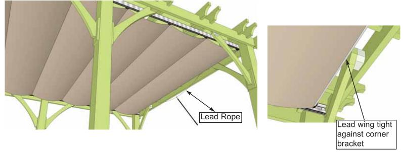
**13.** Pull canopy out using pull handle on lead rope. Fully extend canopy until canopy cannot extend further. Follow **Step 12** to position and attach wing anchor knob to outside girder.
