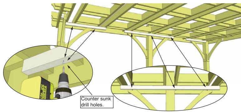
1. With a Step Ladder, install Part A - Canopy Lowering Cleats - 3 pcs Total. (2 pcs. @ 1 1/2" x 2 1/2" x 37 1/4") & (1 pc. @ 1 1/2" x 2 1/2" x 66"). Attach with 2-3 - 4" Torx Screws. Cleats will lower the canopy on one side and drain water off the fabric so it doesn't collect excessively. Decide best side for water to drain for your situation. Position cleats underneath pergola joists or blocking as shown above and attach. Cleats are pre-drilled for Torx Screws.
