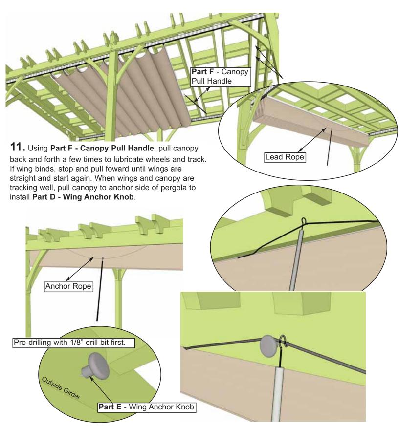
**12.** With canopy pull handle or hand, pull anchor rope up tight so anchor canopy wing is up against inside of pergola bracket. Center Anchor Knob from side-to-side and mark. Before attaching, make sure anchor rope will be snug when slipped over knob. Screw wing anchor knob into outside girder. Pre-drilling with 1/8" drill bit first.
