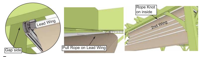
**7.** Before feeding Part C - 109" long Aluminum Wings (8) with Canopy into track, make sure canopy fabric is facing the correct direction. First, locate Lead and Anchor Wings in set. Both have a black pull rope attached. Make sure rope knots are facing to the inside and the pull rope is facing to the outside. Starting with the Lead Wing, feed the wing wheels onto the track as shown above. Wheels have springs and compress in and out slightly to fit.
