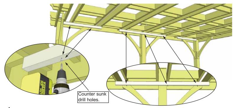
**1.** With a Step Ladder, install **Part A - Canopy Lowering Cleats - 3 pcs Total. (2 pcs. @ 1 1/2" x 3 1/2" x 37 1/4") & (1 pc. @ 1 1/2" x 3 1/2" x 66")**. Attach with **2-3 - 4" Torx Screws.** Cleats will lower the canopy on one side and drain water off the fabric so it doesn't collect excessively. Decide best side for water to drain for your situation. Position cleats underneath pergola joists or blocking as shown above and attach. Cleats are pre-drilled for Torx Screws.
