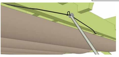
**14.** Extend and contract the canopy several times with pull handle. When extending or contracting the canopy, **pull** firmly in one continuous motion to prevent wings from binding.
