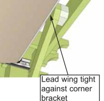
**13.** Pull canopy out using pull handle on lead rope. Fully extend canopy until canopy cannot extend further. Follow **Step 12** to position and attach wing anchor knob to outside girder.
