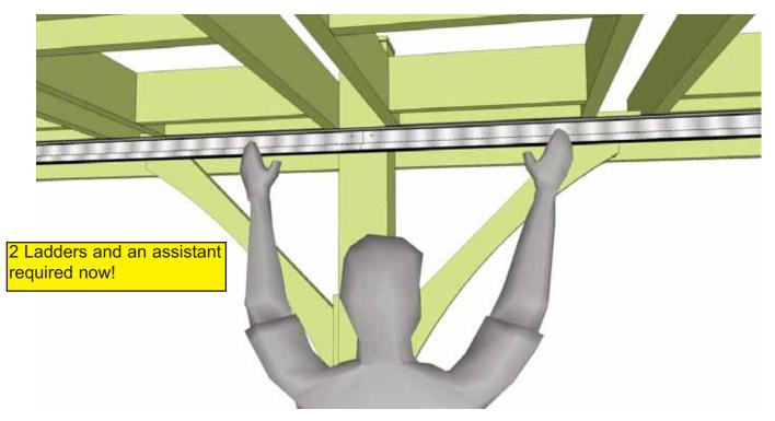
**3.** Carefully lift connected track up supporting in the center. Place tight against post and underneath pergola joists.
