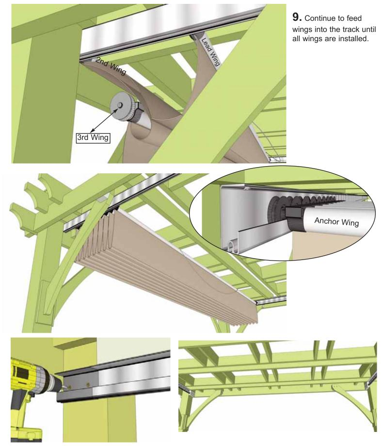
**10.** Install **Part D - 4 1/4" long Aluminum Wing Stops - 2 Pcs.** where track ends and gap exists. Use 2 - 1 1/4" brown screws per stop to install. When removing the wings and canopy in the future, simply remove wing stops and roll wing and canopy out carefully with a helper.
