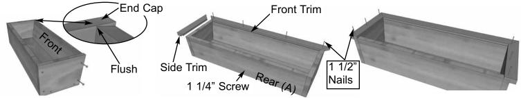
**2.** Position Front Frame Piece flush with End Cap. Attach both ends with 2 - 1 1/4" screws. Pilot hole Rear Box Frame near bottom center and secure to Base edge with 1 - 1 1/4" screw. Evenly position Front Trim (mitre cut on end and dado cut on inside bottom) tight against front frame and nail down with 4 - 1 1/2" nails. Position Side Trims as per Front and secure with 3 - 1 1/2" nails per side.
