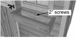
**3.** On a flat surface, flip Flower Box on it's rear face. Evenly space Brackets and secure through Base Frame and into the Brackets with 2 - 1 1/4" screws per Bracket. Position completed Flower Box beneath window trim and screw from inside of box into the center wall stud with 2 - 2" screws. (2" screws supplied with Base Kit.)
