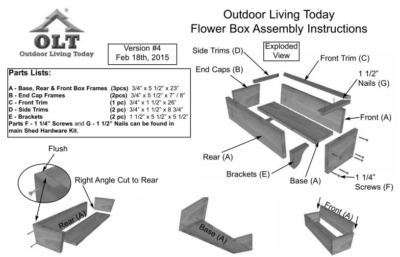
1. On a table position Rear Box and End Cap Frames together so flush at top. Fasten together with
