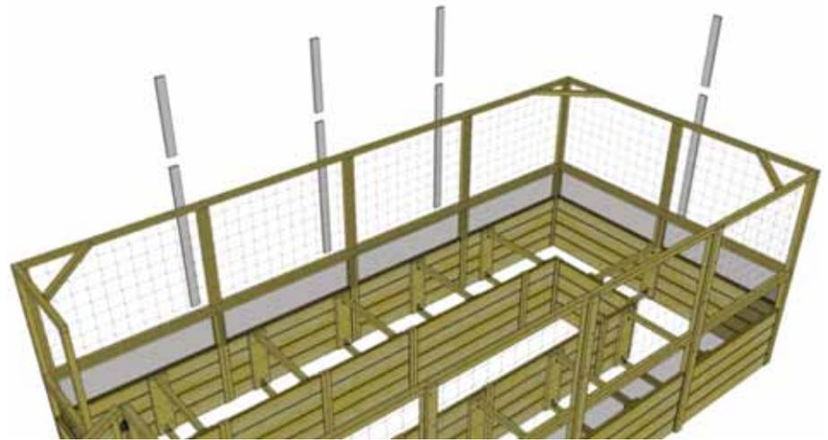
**9.** Position and attach short Vertical Panel Support using **3 - 2" screws** as per **Step 8**. Complete remaining rear and side walls.
