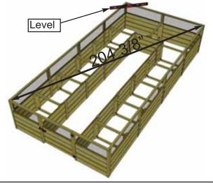
**1.** Prior to installing your Deer Fence Option Kit, confirm your 8x16 Raised Bed is level and square. Measure diagonally inside corner to corner (approximately 204 3/8") in both directions. Adjust as required. Use a level to determine if the tops of the bed frames are sloped and adjust if necessary.
