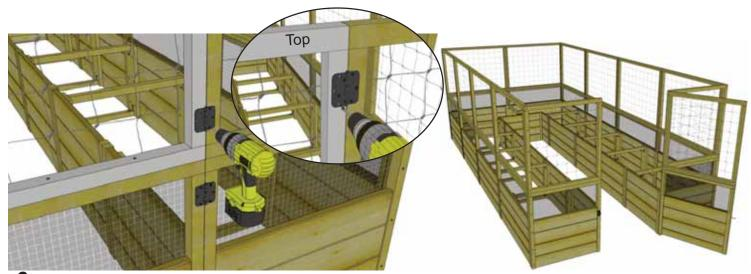
**6.** Locate both **Black Plastic Hinges (3)** and attach to deer fence frame with **6 - 3/4**" **black screws per hinge** as shown above. Use 1/8" drill bit to pilot hole shallow holes before attaching to avoid splitting deer fence framing. Open and close door to check door aligned correctly. Adjust as required.
