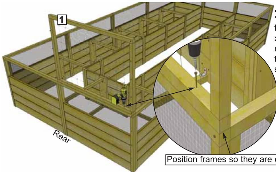
**2.** Starting in rear corner, position the frame of a **Rear Panel (1) - 46" wide x 33 5/8" high** directly on top of the raised bed frame. Screw frames together with **4 - 2 1/2" screws** as shown on the left.
