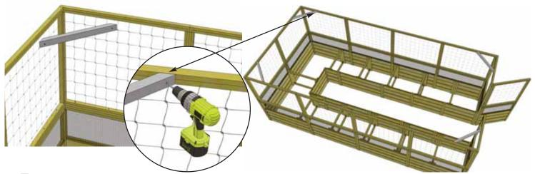
**7.** Attach **Corner Brackets with angle cut ends - (4)** on the inside frames at the top. Use **2 - 2 1/2**" **screws** per bracket. Screw on an angle. Pre-drill ends with 1/8" drill bit to prevent wood splitting.
