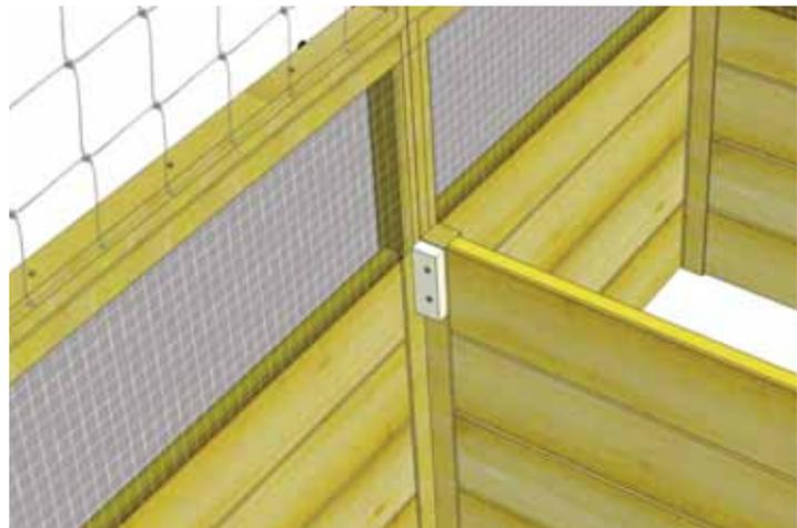
**11.** The **Door Stop (I)** and screws were included with your 8x16 Raised Garden Bed Kit. See **Step 21** of that manual. Install the Door Stop at the top of interior panel frame as shown above.
