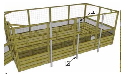
**8.** Locate Vertical Panel Supports - Long (5) - 3/4" x 2 1/2" x 45" and Vertical Panel Supports - Short (6) - 3/4" x 2 1/2" x 22". Starting with 45" long support first, center on panel frames, flush at bottom and attach with 4 - 2" screws. Offset the screw to either side of the support to ensure you contact the heart of the bed frame.
