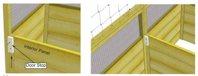
**11.** The **Door Stop (I)** and screws were included with your 8x16 Raised Garden Bed Kit. See **Step 21** of that manual. Install the Door Stop at the top of interior panel frame as shown above.
