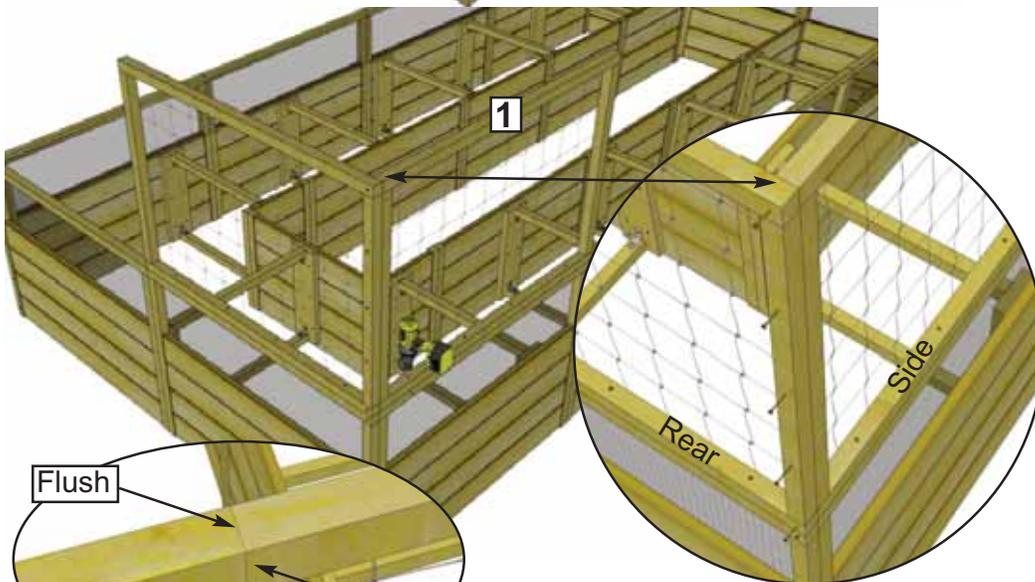
**3.** Position a **Side Panel (1) - 46" wide x 33 5/8" high** directly on top of the side raised bed frame. Hold both deer fence frames together and starting at the top, screw together with **5 - 2 1/2" screws** as shown on the left. Screw bottom of frame down to raised bed frame with **4 - 2 1/2" screws**.
