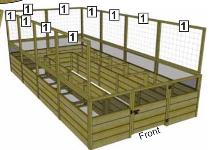
**4.** Position a second **Rear Panel (1) - 46" wide x 33 5/8" high** on top of the rear raised bed frame. Hold both rear deer fence frames together and starting at the top, screw together with **4 - 2 1/2" screws** as shown above. Screw bottom of frame down to raised bed frame with **4 - 2 1/2" screws**. Complete remaining side and rear panels attachments following **Steps 2 and 3**.
