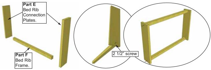
13. To complete rib assembly, locate all 14 Bed Rib Connection Plates (Part E), 12 Bed Rib Frames (Parts F) - 1 1/2" x 1 1/2" x 26 3/8" and 2 longer Bed Rib Frames (Part G) - 1 1/2" x 1 1/2" x 29 1/4". On a level flat surface, screw connection plate and frame together with 1 - 2 1/2" Screw per end. Align so plate and frame are flush at bottom. Complete both sides.
