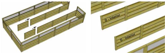
**12.** Align and attach final side **Interior Panels (Part D)** as per **Step 10**. Angle screw panels together with **3 - 2 1/2" Screws** from the inside.
