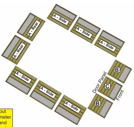
Before positioning panels, lay out footprint and level ground perimeter. If possible, dig a small trench and backfill with 1 or 2 inches of sand. Sand will make it easier to level panels.
