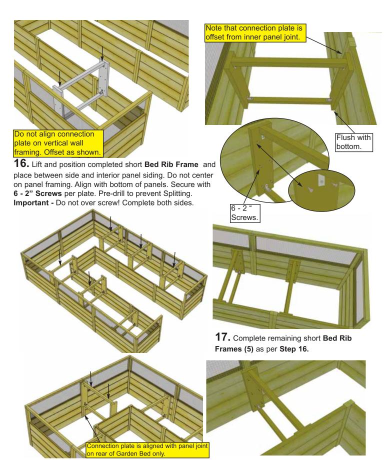
**18.** Lift and center completed longer **Bed Rib Frame** on rear and end interior panels. Align with bottom of panels. Secure with **6 - 2" Screws** per plate. **Important -** Do not over screw!
