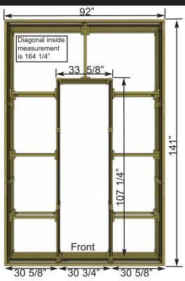
Lay down a sand perimeter base for the Garden frames to sit on if possible. Sand offers excellent drainage and will make it easier to level bed frames.
