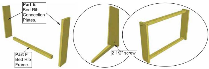
14. To complete rib assembly, locate all 18 Bed Rib Connection Plates (Part E), 16 Bed Rib Frames (Parts F) - 1 1/2" x 1 1/2" x 26 3/8" and 2 longer Bed Rib Frames (Part G) - 1 1/2" x 1 1/2" x 29 1/4". On a level flat surface, screw connection plate and frame together with 1 - 2 1/2" Screw per end. Align so plate and frame are flush at bottom. Complete both sides.
