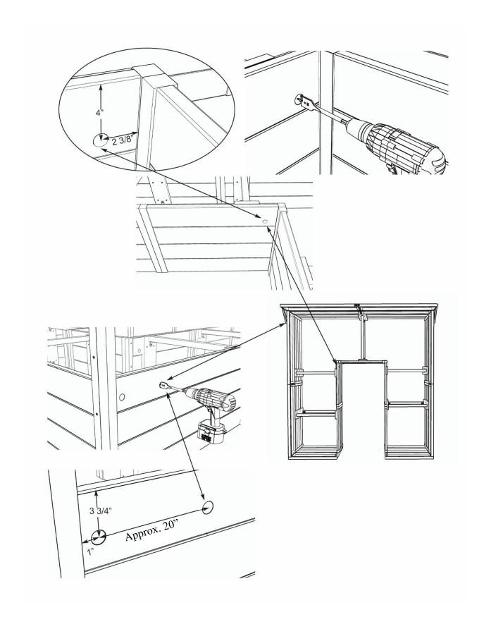
**Step 3** – Start with the interior panel first, with a ¾" Spade Bit, drill 4" down and 2 3/8" from the end, as shown at the top of the illustration on this page. Now drill the outside panel holes following the lower part of the illustration on this page. One hole will be drilled 1" from the inside of the 2x2 frame and second is approximately 20" from that mark. Hole location is important so mark holes first with a pencil and then hold the timer assembly up to confirm.
